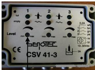
Turn external potentiometer in direction of the arrow to "12 o'clock" position
