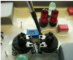
Adjust the switching point by turning the internal (20-pitched) potentiometer!
