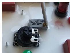
Adjust the switching point by turning the internal (20-pitched) potentiometer!
